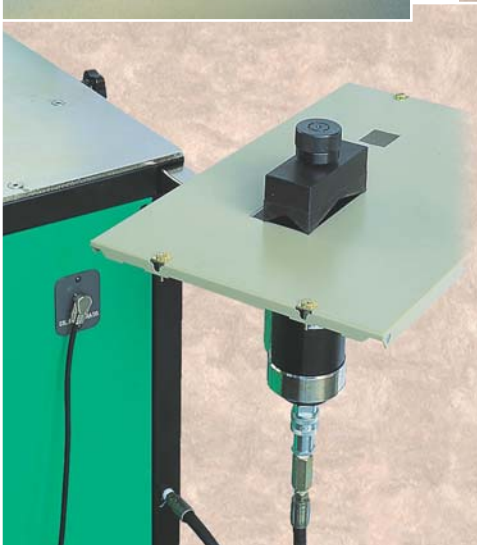
FORA - PANNELLI ELECTRICAL PANEL BOARD DRILLING
