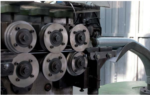
Profilatrice tubo flessibile Roll forming machine for flexible conduits
